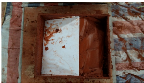
图 5 插入雪弗板的试块 Fig.5 A sample with Shaver board
