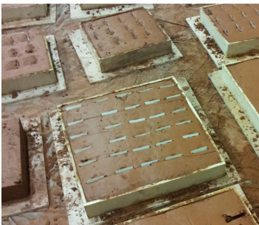
Fig. 7. Prefabricated blocks and Teflon tape.
